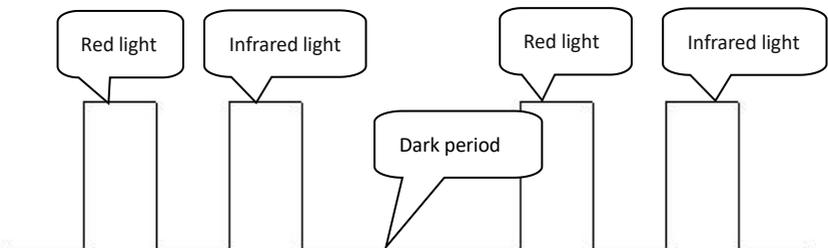
3, red and infrared light continuous light, no dark interval in the middle or dark interval is very small, less than 100us, as shown in the following figure:
