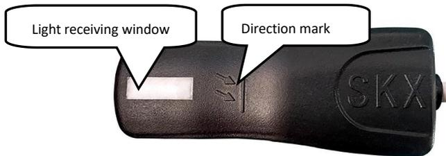
Place this side of the simulated finger (shown above) on the red tube end of the blood oxygen probe
