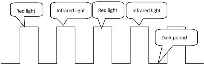
2, The timing of red and infrared light is fixed, as shown in the figure below:
