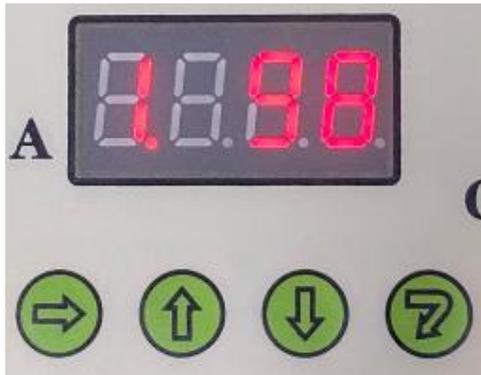
As shown in the figure above, the current display content of the digital tube is 1.98, and there is a red decimal point in the lower right corner of the digital tube of the number 1, which represents the current number as the changeable item of the menu option;
