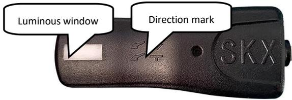
Place this side of the simulated finger (shown above) on the receiving tube end of the blood oxygen probe
